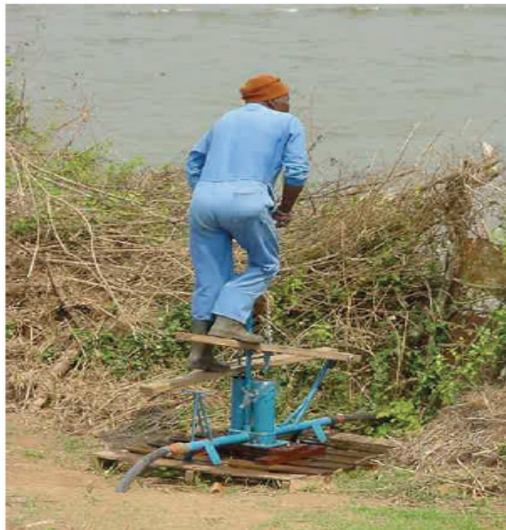
Figure 12-4 A Zambian farmer pumping water with a pressure treadle pump (Kedge, 2001)
